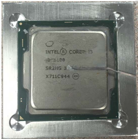
Intel Core i3 processor with thermocouple embedded in the lid
