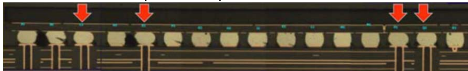
Cross-section of a BGA array (left) with solder separation defects (above) seen to occur at VIPPO locations.
