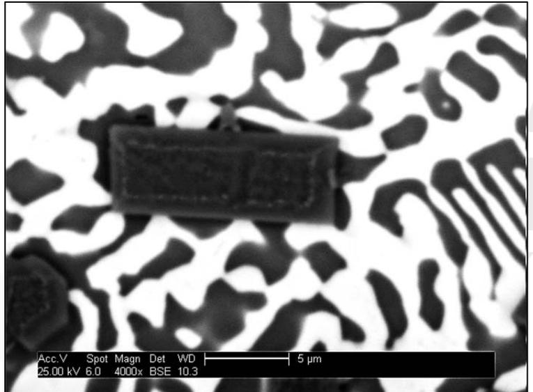
(a) Bright field image of 57Sn42Bi1Ag solder joint on Cu-OSP board finish and 60s TAL reflow. (b) Cross polarized image of the same joint, and (c) an SEM image of the eutectic lamellae with a Sn rich (dark) phase and Bi rich (light) phase. Blocky third phase particles are seen throughout.
