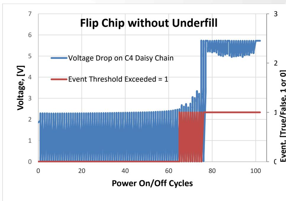
*Output of tandem failure detection circuits in the power cycle system for a flipchip solder joint circuit. Analog test net voltage drop (blue) corresponds well with digital event detection signal (red).*
