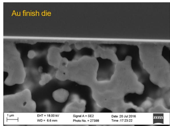
*Sintering of silver paste against a silver finish die (LEFT) produces a robust layer of dense silver at the interface. This dense layer is absent on the gold finish die (RIGHT) despite an identical sintering schedule.*
