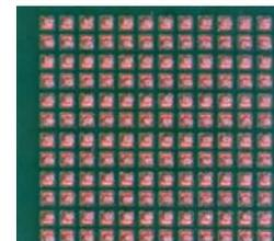
Left: Sample results from KohYoung SPI tool illustrating transfer efficiency for various stencil types. Right: Visual images of paste deposits are also being captured to reveal qualitative print differences.
