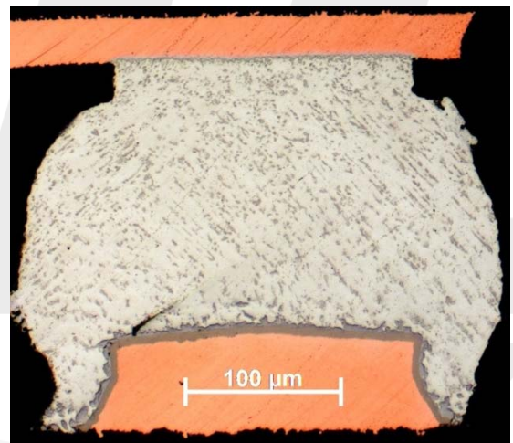
Bright field image of a 10 mil solder ball of the 'Violet' alloy composition (Sn2.25%Ag0.5%Cu6.0%Bi) on an ENIG surface board.
