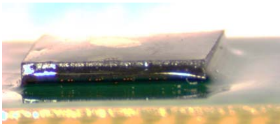
UV40 coating fully encapsulates bottom terminated components such as this QFN.
