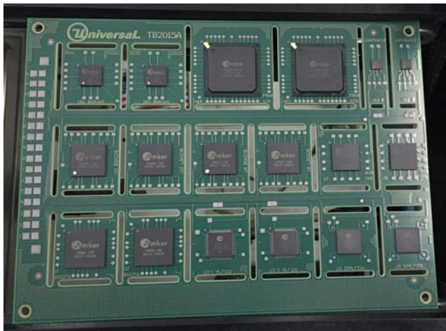
Assembled TB2015 test board used in the alternate alloy study; various LGA, BGA and MLF package types are being tested.
