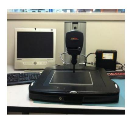
Application: Endoscopic optical inspection of wire bonds, BGAs, through-holes, J-legs, gullwings, leaded heel fillets, solder paste and adhesive deposits and height measurements.
