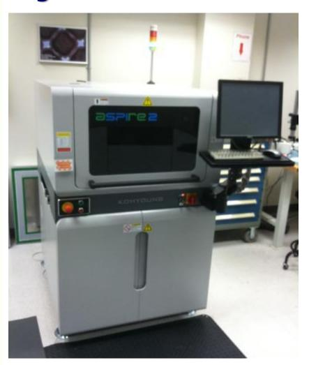
Application: 3-D solder paste inspection of volume, area, height, offset, bridging, shape deformity, coplanarity
